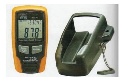
This data logger module can be used to monitor humidity and temperature of greenhouses, warehouses, food transports, aircraft cabins, refrigerated trucks, containers, museums, and HVAC equipment.
