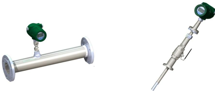
**MYKO** Thermal mass flow meter is designed on the basis of thermal dispersion, and adopts method of constant differential temperature to measuring gas flow. It has advantages of small size, easy installation, high reliability and high accuracy, etc
